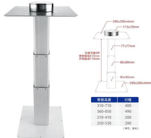
SDTTM-03 手动式榻榻米升降机 (小铝) Manual tatami lift (small aluminum)
